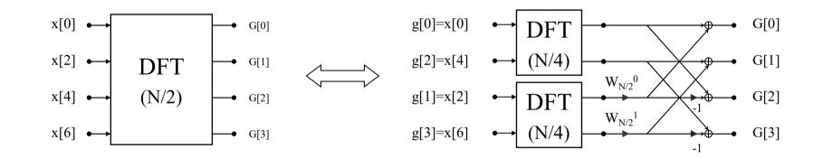
→ its computational cost (multiplications) is proportional to  $2(N/4)^2+N/4 = N^2/8+N/4$ , making that if this structure is used in the computation of G[k] and H[k], the total computational cost (multiplications) involved in the computation of X[k] is proportional to  $2 \times N^2/8+2N/4+N/2 = N^2/4+N$ .
